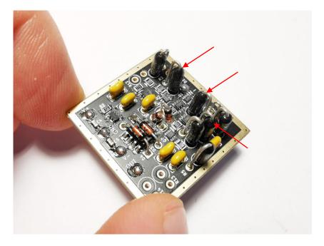
And finally, solder the remaining two big resistors (R13, R14). They are either black 22ohm in the original version or brown 10ohm in the enhanced version.
