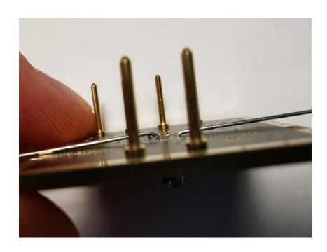
Now clip the first lead in such a way, that the remaining lead overhangs and acts like an anchor for the part and keeps it nice in place, then solder it:
