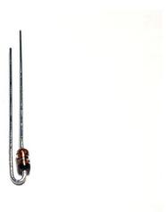
Insert the diodes into D5 and D6 as in the next picture. Then bend its leads as close to the underside of the PCB as possible, to get a tight fit.
