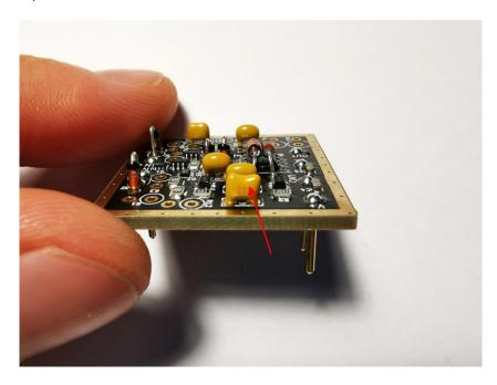
Now solder the last capacitor, it's the 27pF (C8), marked with 270. The location is right behind the 47pF C1 again.
