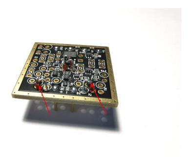
Now take the last two diodes for D3 and D4. They will be strapped across the large SOIC chip. To do this, bend both leads of the first diode so that it will fit into the D3 marking, across the chip. Make the black band of the diode face towards the next chip above. Make also sure, that the diode is strapped across one half of the chip and making contact with it. Solder it in the same manner as before and make sure the position and contact remains.
