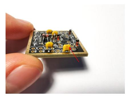
Follow up with the 150pF (C3) capacitor. It's marked with 151 and is located across the board from where the last 22pF was soldered.
