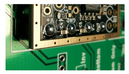
• In case you don't have an existing socket you can or want to use, you can flip the PCB on its back and due to the fact that the SMD transistors are already soldered on, it will rest enough above ground to be able to solder the pins from the bottom:
