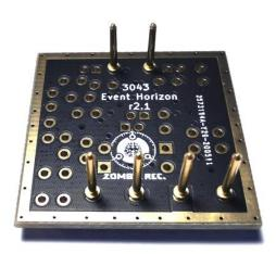
Make sure to heat the pins and the contact surface for a few seconds by gently pushing the soldering iron onto the pin edge and the contact surface on the PCB, then apply enough solder for it to flow to the other side of the PCB.
