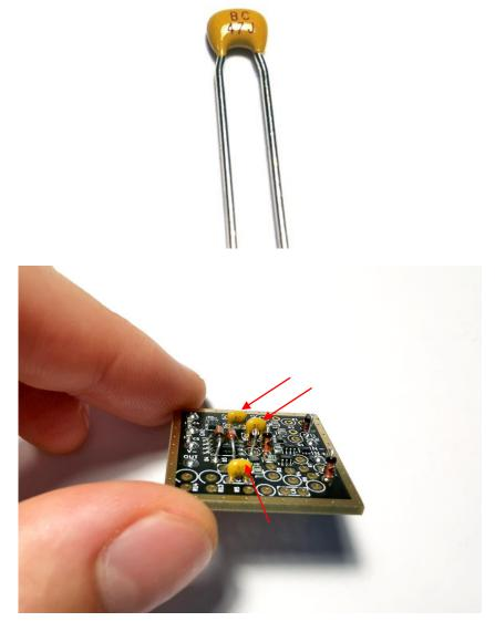
Then solder the 22pF (C6, short leads) capacitor. It's marked with 22J and it is located right next to the 47pF C1. Again, orientation does not matter for all the capacitors.
