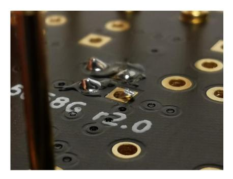
Now the next two diodes for soldering D1 and D2 at the front. Check the image below on how to insert them (black band towards the white silkscreen ring). They are located at the edge of the PCB. Solder them the same way as described before.
