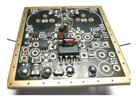
Now do the same thing for the last diode D4. **Make it face the other direction than D3 does!**Place the second diode properly above the other half of the chip and make sure it has contact.
